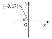
b  $\tan \theta = \frac{17}{9} \implies \theta = 1.084 \dots$ z is in the second quadrant.  $\arg z = \pi - 1.084 \dots = 2.057 \dots$ = 2.06, in radians to 2 d.p. You have to give your answer to 2 decimal places. To do this accurately you must work to at least 3 decimal places. This avoids rounding errors and errors due to premature approximation.
