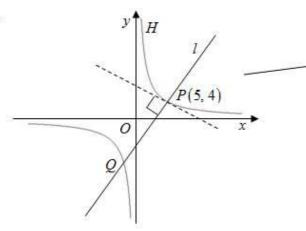
The normal to H at P is perpendicular to the tangent at P. The tangent has here been drawn as a dotted line. To work out perpendicular gradients you will need the formula mm' = -1.
