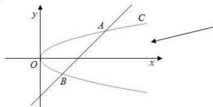
You have to recognise that  $x = 3t^2$ , y = 6t is a parabola and draw it passing through the origin with the correct orientation.
